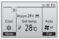
will appear on the Main display in the Full mode when the operation lock function setting is enabled.
